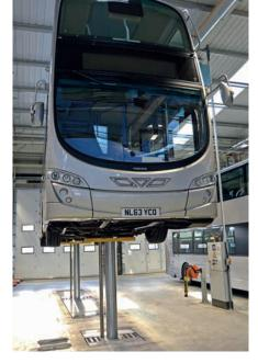
vulnerable to the risk of the lifted vehicle overturning, since their weight may not always be spread evenly between the left and right sides. To ensure that overturning can't happen, Totalkare two-post lifts have wire ropes attached between both lift arms to keep them operating in a synchronised manner, regardless of the vehicle's lateral balance.
